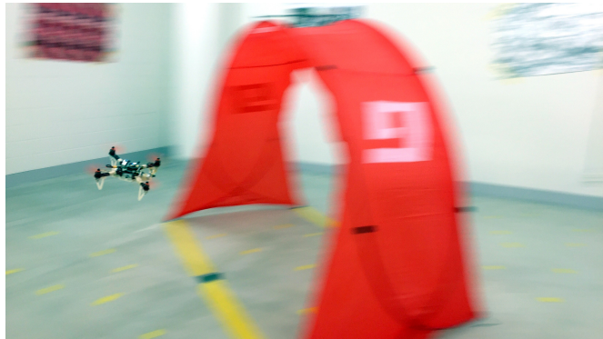
Fig. 1: By combining a convolutional neural network with trajectory generation and control methods, our vision-based, autonomous quadrotor is able to successfully fly through race tracks with high agility.
