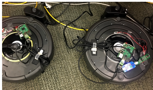
Fig. 1: Two iRobot2 [4], equipped with two RPi3s [5].
